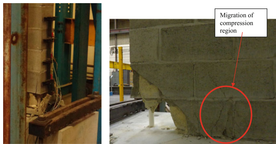
Fig. C.18 Flexural failure of wall W4
