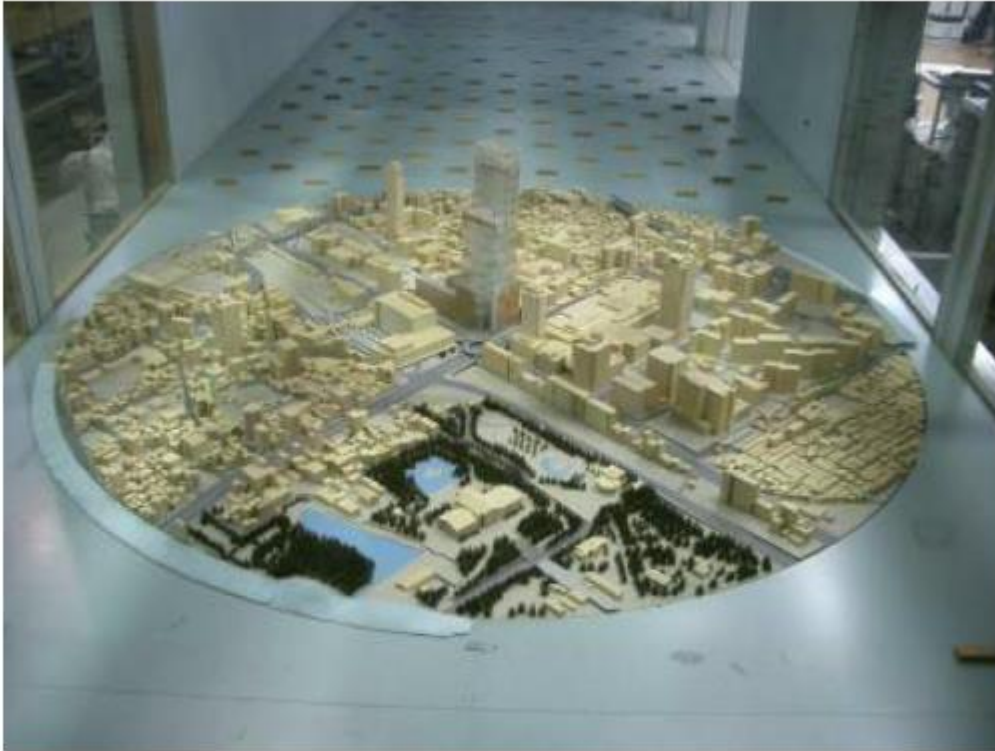
Figure 4. Wind tunnel test model.
