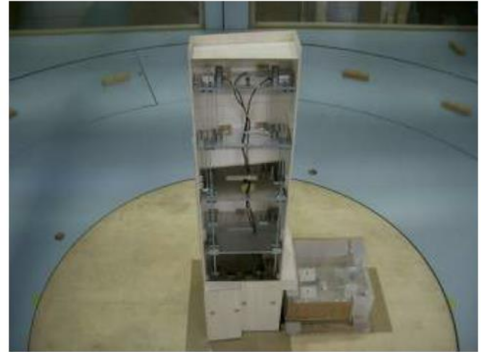
Figure 8. Aerodynamic vibration test using MDOF model.
