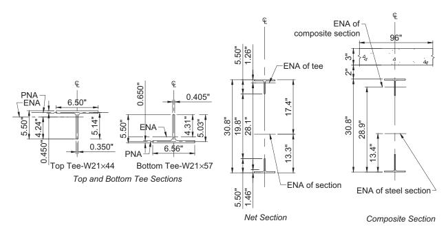
Fig. 4-6. Tee, net and composite sections for castellated beam for Example 4.3.
