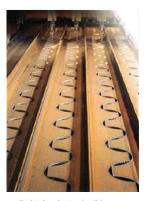
Fig. 1-4. Second cutting of a cellular pattern.
