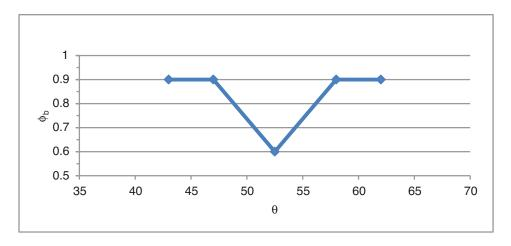
Fig. 3-8. Resistance factor by hexagonal cut angle.
