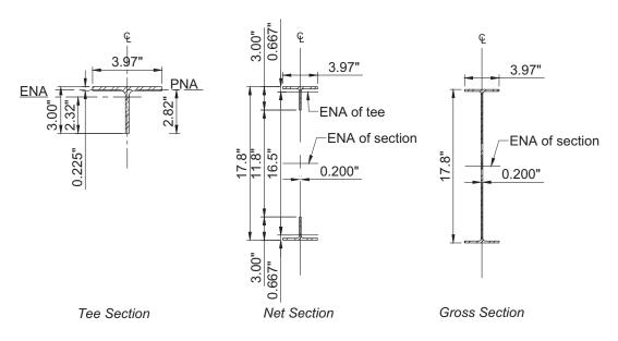
Fig. 4-2. Tee, net and gross sections of castellated beam for Example 4.1.
