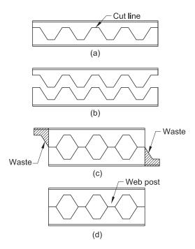
Fig. 1-1. Manufacturing of a castellated beam.
