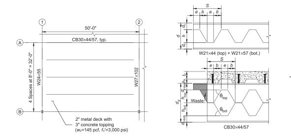
Fig. 4-5. Structural framing layout and composite castellated beam nomenclature for Example 4.3.
