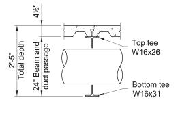
Fig. 2-4. 14-in.-diameter HVAC duct.
