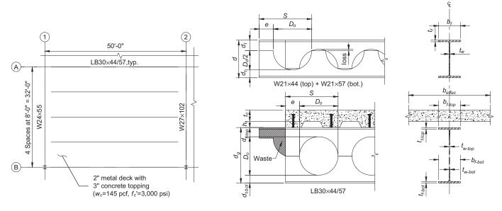
Fig. 4-7. Structural framing layout and composite cellular beam nomenclature for Example 4.4.
