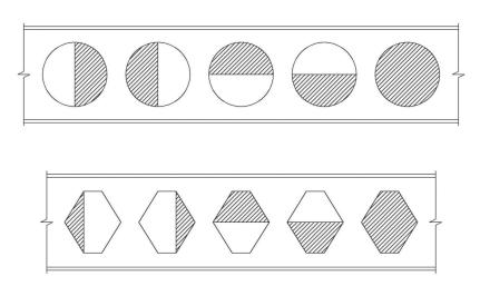
Fig. 2-10. Typical infill patterns for cellular (top) and castellated beams (bottom).
