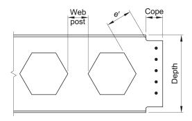
Fig. 2-12. Minimum distance between the end cope and the first opening, e'
