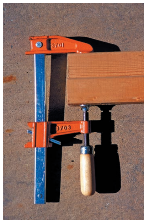
Photo 4.2 Clamp used to glue lumber pieces together.
