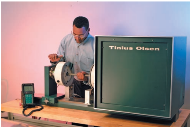
Photo 3.3 Tabletop torsion testing machine.
