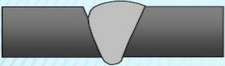
Incomplete filled groove + Lack of sidewall fusion
