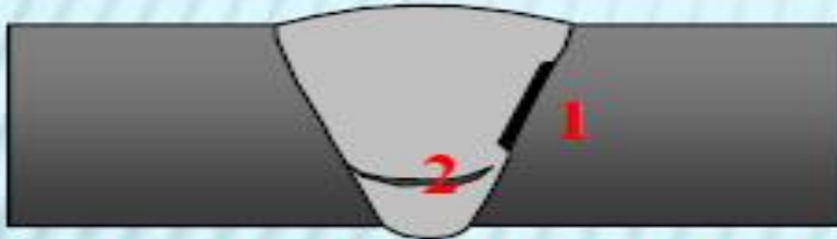
Incomplete filled groove + Lack of sidewall fusion
