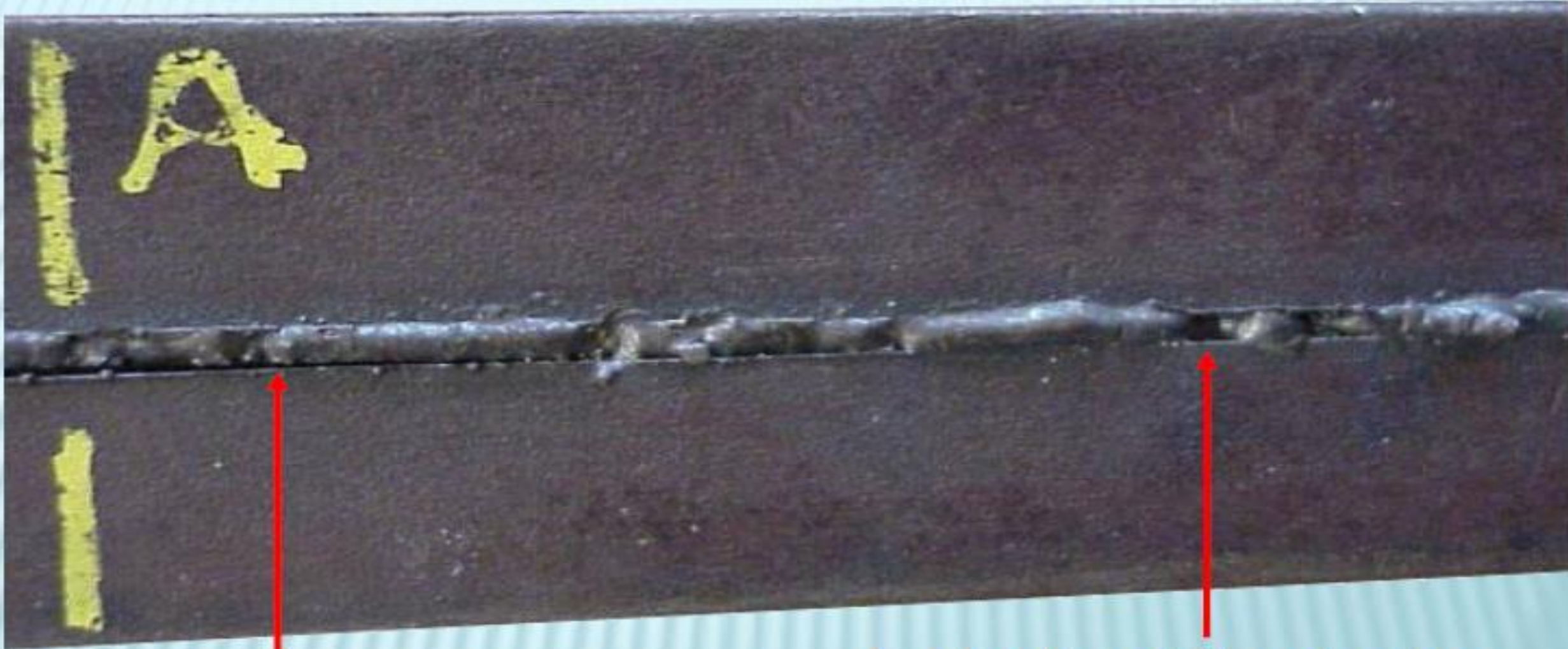
Lack of root Penetration
