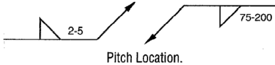
Figure 4.65—Length, Pitch Fillet Welds
