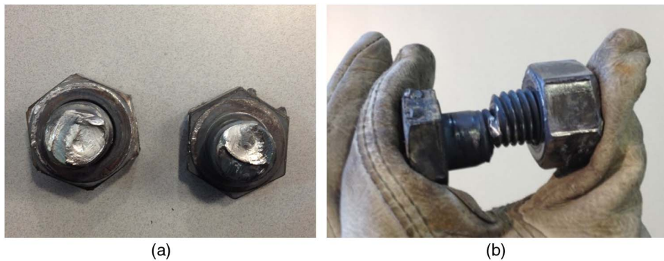
Fig. 5. Bolt shear fracture for Specimen BS-3 (400°C): (a) profile view of shear fracture of bolt; (b) fracture surface of bolt after experiment
