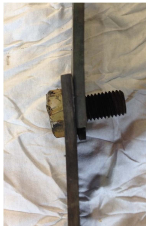
Fig. 9. Cross section through lap-splice joint of Specimen 2-PB-400
