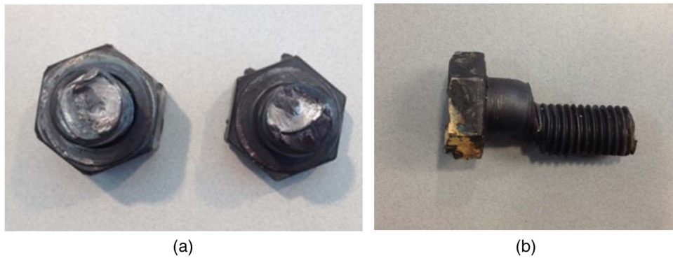
Fig. 6. Bolt shear fracture for Specimen BS-4 (600°C): (a) profile view of shear fracture of bolt; (b) fracture surface of bolt after experiment
