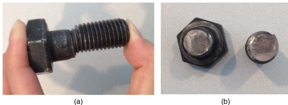
Fig. 4. Bolt shear fracture for Specimen BS-1 (ambient temperature): (a) profile view or shear fracture of bolt; (b) fracture surface of bolt after experiment
