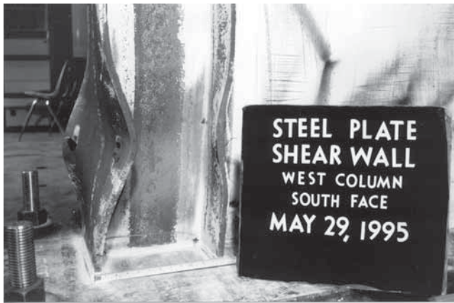
Fig. 2–26. Local buckling and fracture of column at end of test (courtesy of Robert Driver, University of Alberta, Edmonton, Canada).
