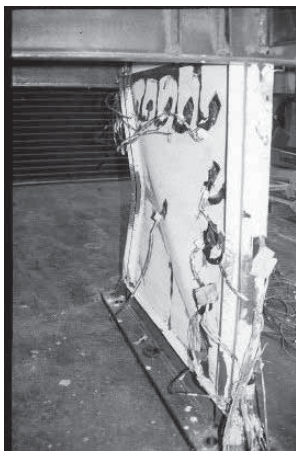
Fig. 2-34. Near and far view of local instability of columns at first story of SPW (courtesy of Carlos Ventura, University of British Columbia, Vancouver, Canada).
