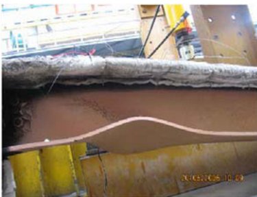
Fig. 7.8 Local buckling of the restrained beam
