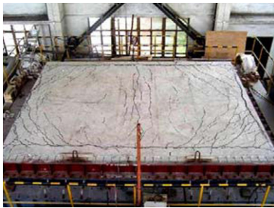
Fig. 9.23 Cracks on the S-2 after the test
