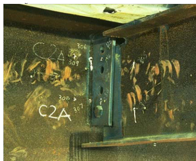
(c) Fracture of the beam to column joint
