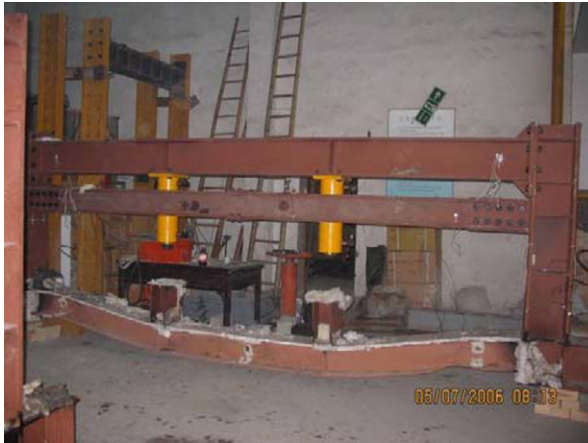
Fig. 7.7 Deflection of the restrained beam
