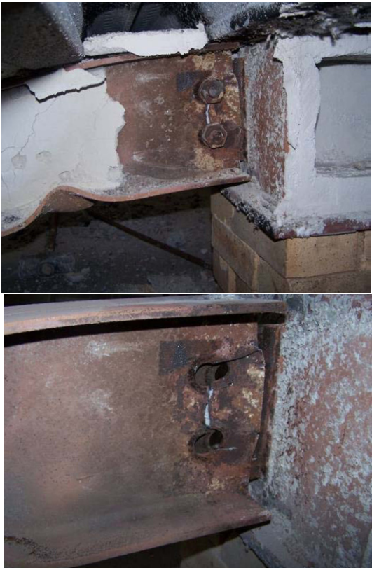
Fig. 7.40 Breaking of the joint in test CB150
