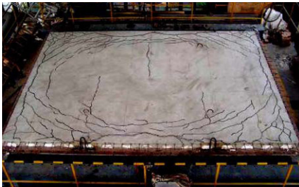
Fig. 9.26 Cracks on S-3 after the test
