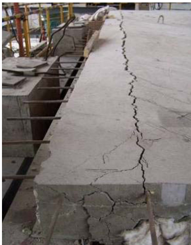
Fig. 9.19 Cracks along the long edge on S-1
