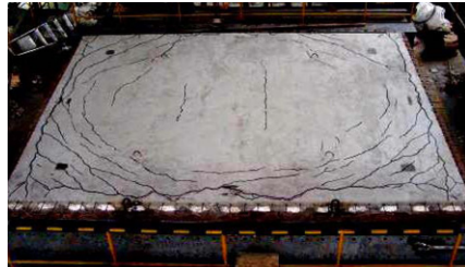
Fig. 9.27 Cracks on S-4 after the test
