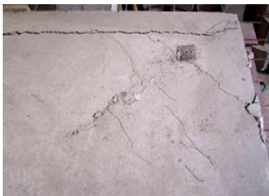
Fig. 9.21 Yield lines at the corner on S-1
