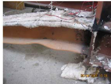
Fig. 7.8 Local buckling of the restrained beam
