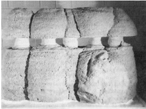
**FIGURE 13.32** Grout curtain in stratified deposits made with single row or holes.
