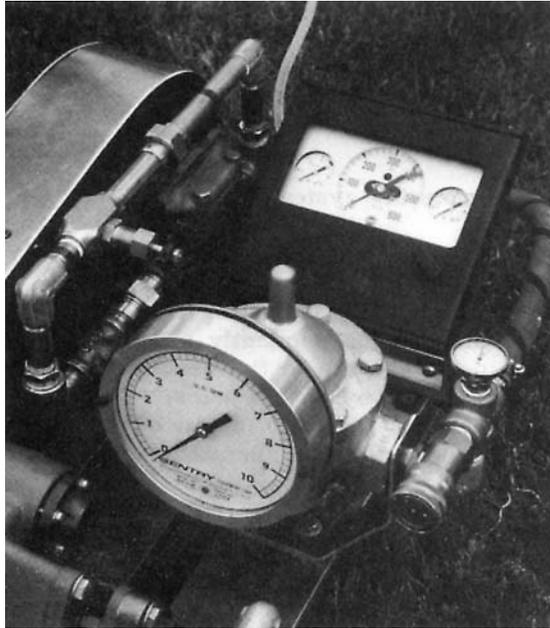
**FIGURE 14.5** Chemical grout metering system.
