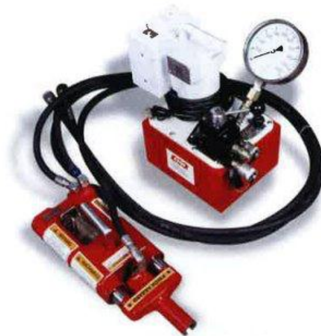
FIGURE 2.4.3A-1 Equipment for Mono-Strand Stressing (P158)
