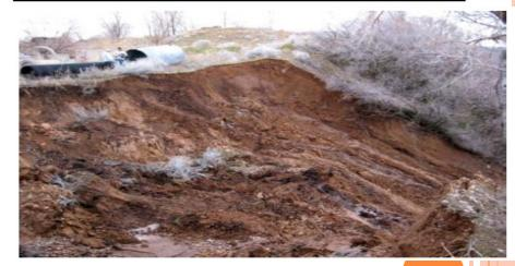
b) Translational slides occurs when the failure surface is approximately flat or slightly undulated
