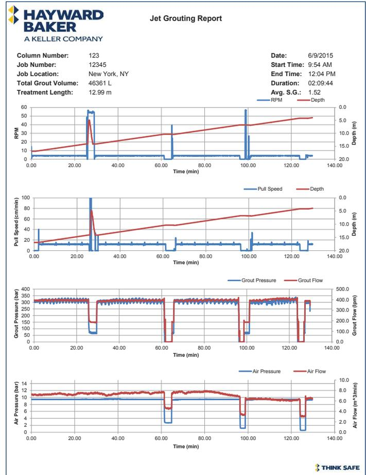
HBI DAQ report for a jet grout column. The report is specifically designed for a quick, one page overview of the jet grout installation.
