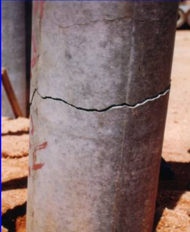
Seriously damaged pile due to severe driving stress in soft ground (tension)
