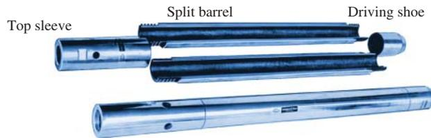
Fig. 2.7 Illustration of a split spoon sampler.
