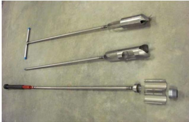
**Fig. 2.3** Hand auger and sampler.
