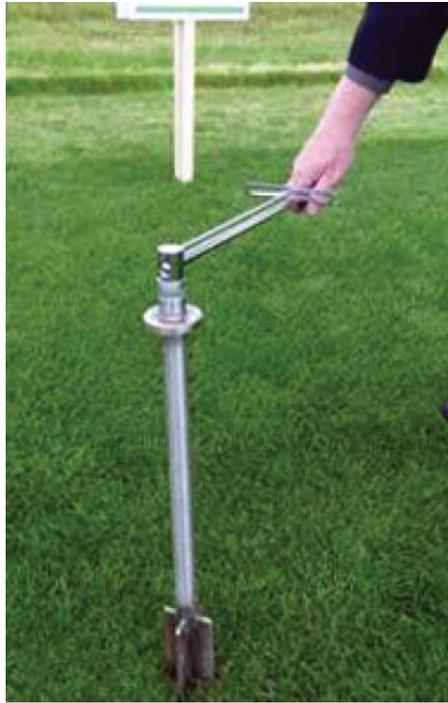
Fig. 2.15 Vane shear test.
