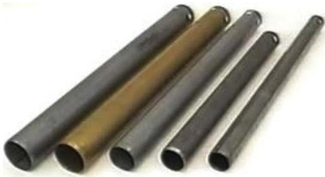
**Fig. 2.9** Shelby tube sampler.
