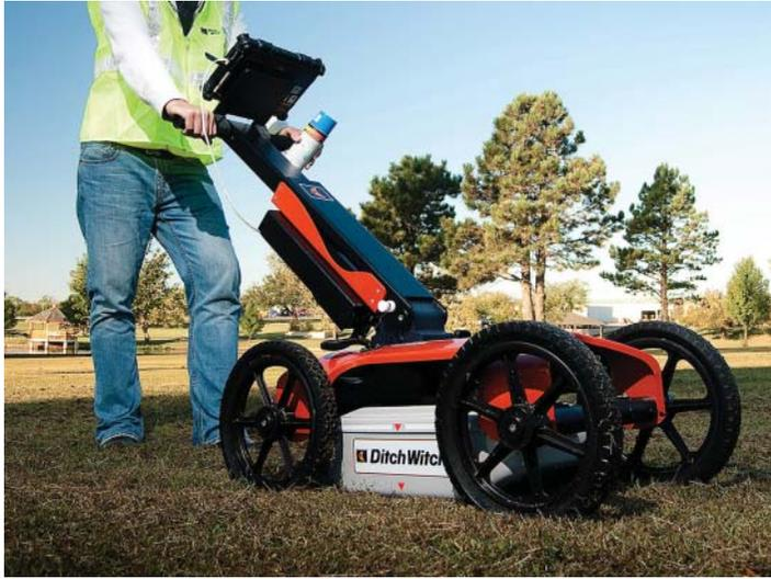
**Fig. 2.20** Hand-operated GPR. (Photo courtesy of Charles Machine Works, Inc.)
