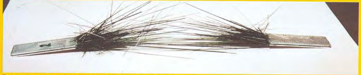
Sample after loading with failure load
