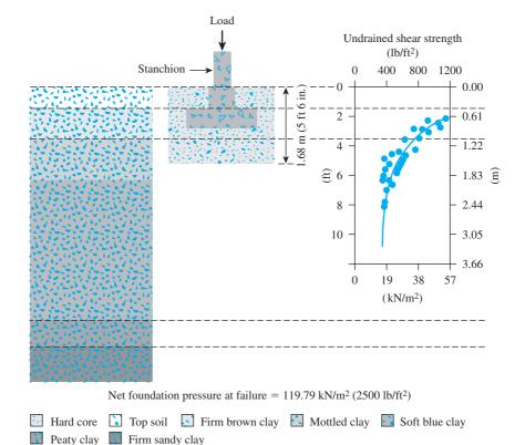
Figure 16.11 Skempton's field-load test on a foundation supported by a saturated clay (After Bishop and Bjerrum, 1960. With permission from ASCE.)
