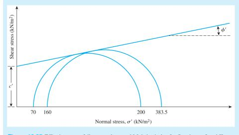
Figure 12.25 Effective stress failure envelope and Mohr's circles for Specimens I and II
