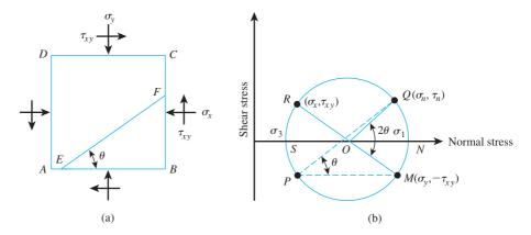
*Figure 10.5* (a) Soil element with normal and shear stresses acting on it; (b) use of pole method to find the stresses along a plane
