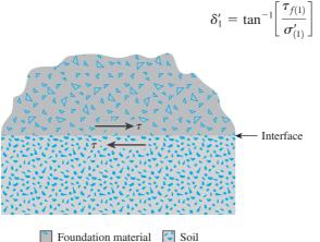
**Figure 12.13** Interface of a foundation material and soil
