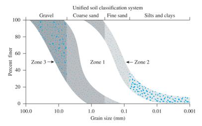
Figure 6.34 Effective range of grain-size distribution of soil for vibroflotation
