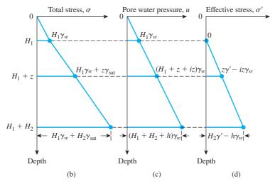
Figure 9.4 (a) Layer of soil in a tank with upward seepage. Variation of (b) total stress; (c) pore water pressure; and (d) effective stress with depth for a soil layer with upward seepage
