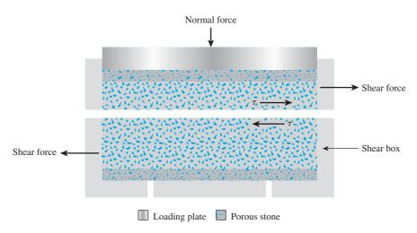
Figure 12.4 Diagram of direct shear test arrangement
