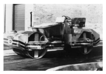
Figure 6.15 Smooth-wheel roller (Ingram Compaction LLC)
