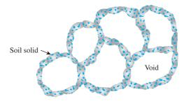
Figure 4.20 Honeycombed structure
