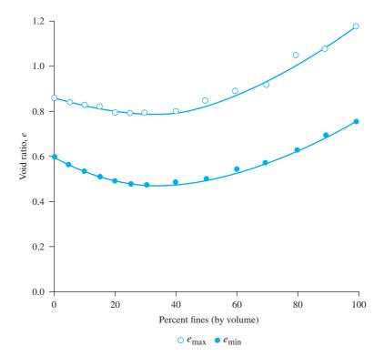
Figure 3.8 Variation of  $e_{\text{max}}$  and  $e_{\text{min}}$  (for Nevada 50/80 sand) with percentage of non-plastic fines (Redrawn from Lade et al, 1998. Copyright ASTM INTERNATIONAL. Reprinted with permission.)
