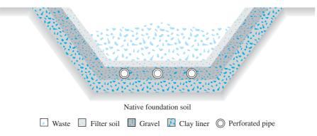
Figure 17.8 Cross section of single clay liner system for a landfill
