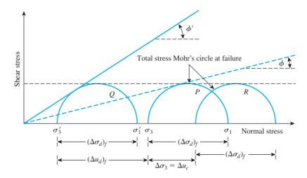
**Figure 12.32** The  $\phi = 0$  concept
