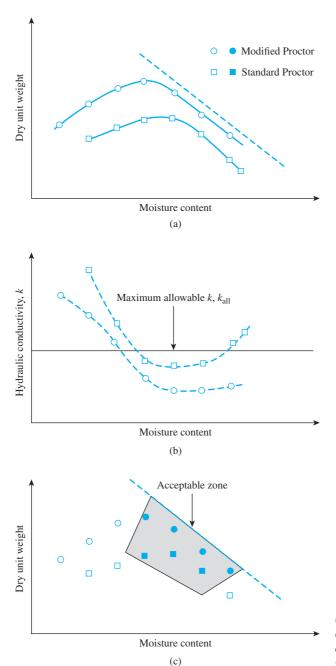
**Figure 17.3** (a) Proctor curves; (b) variation of hydraulic conductivity of compacted specimens; (c) determination of acceptable zone
