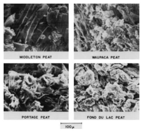
Figure 5.8 Scanning electron micrographs for four peat samples (After Dhowian and Edil, 1980. Copyright ASTM INTERNATIONAL. Reprinted with permission.)
