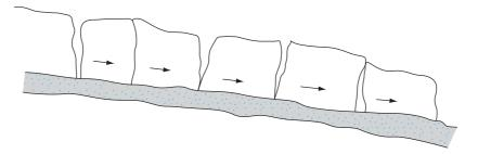
Figure 15.5 Slope failure by lateral "spreading"
