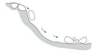
Figure 15.1 "Fall" type of landslide
