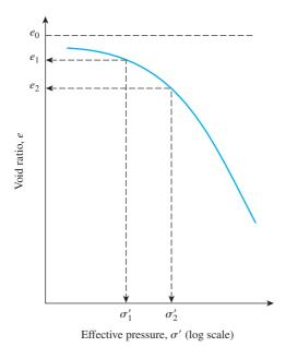
**Figure 11.10** Typical plot of e against  $\log \sigma'$
