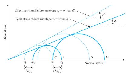
*Figure 12.27* Total and effective stress failure envelopes for consolidated undrained triaxial tests. (*Note:* The figure assumes that no back pressure is applied.)
