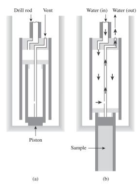
**Figure 18.9** Piston sampler: (a) sampler lowered to bottom of borehole; (b) pressure released through hole in piston rod
