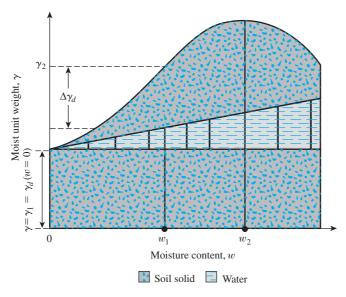
Figure 6.1 Principles of compaction
