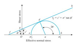
Figure 12.3 Mohr's circle and failure envelope
