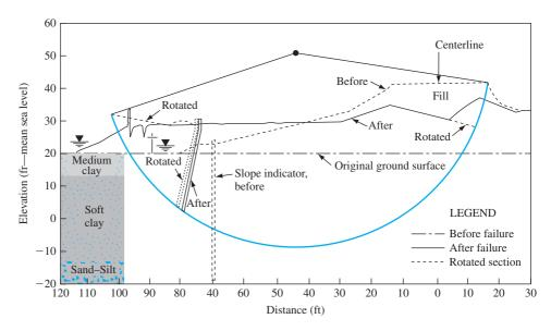
*Figure 15.39* Cross-section of the experimental test section before and after failure (*After Ladd, 1972. With permission from ASCE.*)
