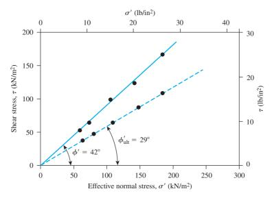
Figure 12.9 Determination of shear strength parameters for a dry sand using the results of direct shear tests
