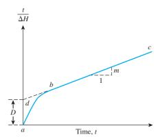
**Figure 11.27** Hyperbola method for determination of  $c_v$
