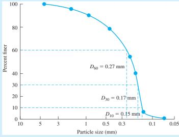
Figure 2.28 Particle-size distribution curve
