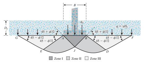
Figure 16.10 Soil-bearing capacity calculation—general shear failure
