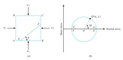
**Figure 10.3** (a) Soil element with AB and AD as major and minor principal planes; (b) Mohr's circle for soil element shown in (a)
