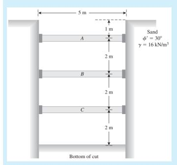
Figure 14.13 Braced cut in sand
