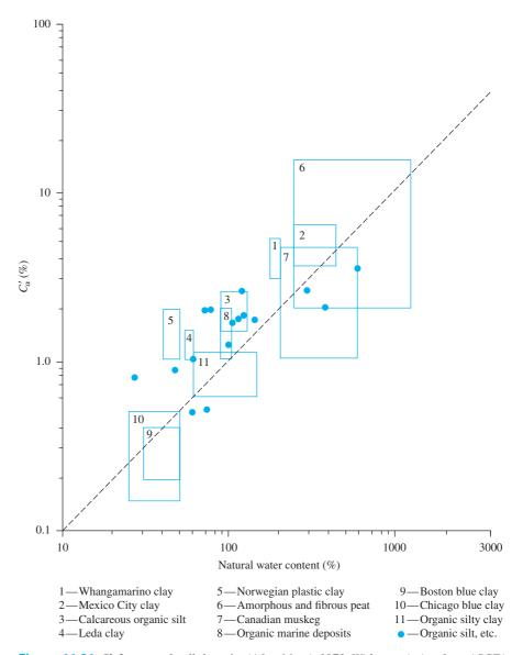
**Figure 11.21**  $C'_{\alpha}$  for natural soil deposits (After Mesri, 1973. With permission from ASCE.)
