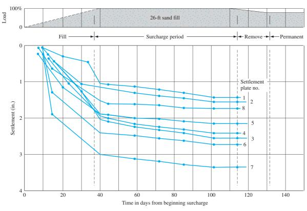
Figure 11.34 Settlement-time curves beneath the surcharge fill area for the construction of Tampa VA Hospital (After Wheelen and Sowers, 1972. With permission from ASCE.)
