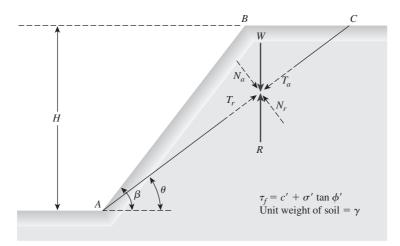
Figure 15.10 Finite slope analysis-Culmann's method
