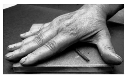
Figure 4.7 Rolling of soil mass on ground glass plate to determine plastic limit (Courtesy of Braja M. Das, Henderson, Nevada)
