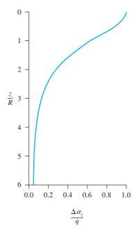
**Figure 10.18** Stress under the center of a uniformly loaded flexible circular area
