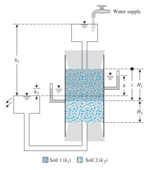
Figure 8.2 Flow through a two-layered soil
