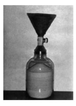
Figure 6.22 Glass jar filled with Ottawa sand with sand cone attached (Courtesy of Braja M. Das, Henderson, Nevada)
