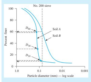
Figure 5.7 Particle-size distribution of two soils
