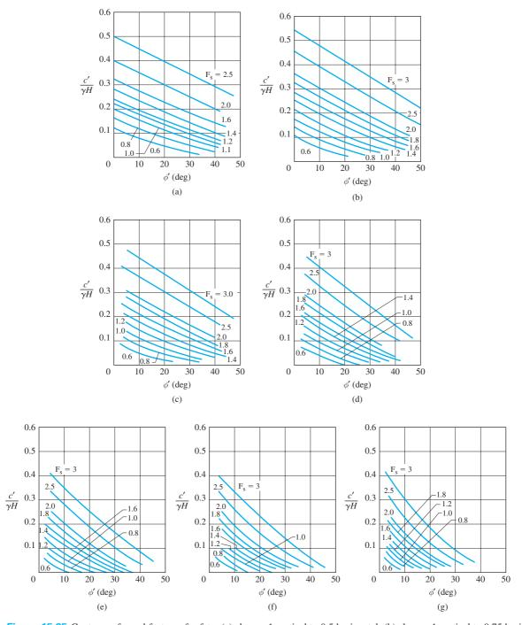
**Figure 15.25** Contours of equal factors of safety: (a) slope – 1 vertical to 0.5 horizontal; (b) slope – 1 vertical to 0.75 horizontal; (c) slope – 1 vertical to 1 horizontal; (d) slope – 1 vertical to 1.5 horizontal; (e) slope – 1 vertical to 2 horizontal; (f) slope – 1 vertical to 2.5 horizontal; (g) slope – 1 vertical to 3 horizontal (*After Singh, 1970. With permission from ASCE.*)
