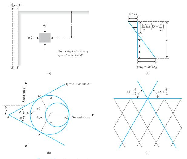
Figure 13.7 Rankine's active earth pressure
