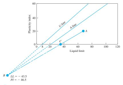
Figure 4.17 Estimation of shrinkage from plasticity chart (Adapted from Holtz and Kovacs, 1981)
