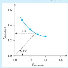
Figure 15.37 shows a plot of  $F_{s(assumed)}$  against  $F_{s(calculated)}$ , from which  $F_s \simeq 1.3$ .
