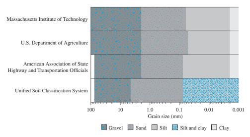
Figure 2.7 Soil-separate-size limits by various systems
