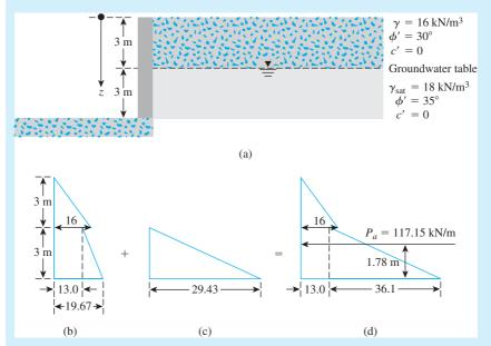
Figure 13.19 Retaining wall and pressure diagrams for determining Rankine's active earth pressure. (*Note*: The units of pressure in (b), (c), and (d) are kN/m<sup>2</sup>)
