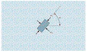
Figure 12.41 Strength anisotropy in clay
