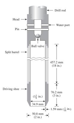
Figure 18.5 Diagram of standard splitspoon sampler
