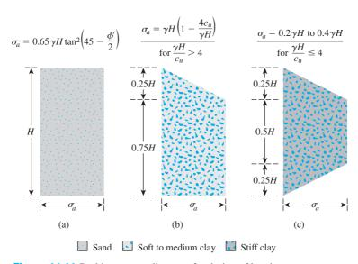
Figure 14.11 Peck's pressure diagrams for design of bracing systems
