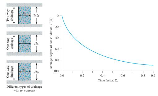
Figure 11.24 Variation of average degree of consolidation with time factor,  $T_v$  ( $u_O$  constant with depth)
