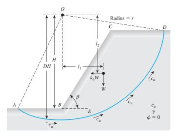
Figure 15.18 Stability analysis of slope in homogeneous saturated clay with earthquake forces  $(\phi = 0 \text{ condition})$
