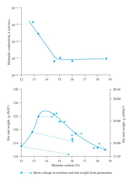
*Figure 6.11* Effect of compaction on hydraulic conductivity of clayey soil (*Redrawn after Lambe, 1958b. With permission from ASCE.*)
