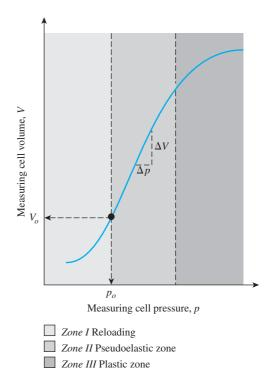
**Figure 18.12** Relationship between measuring pressure and measuring volume for Menard pressuremeter
