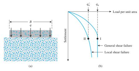
Figure 16.2 Ultimate soil-bearing capacity for shallow foundation: (a) model footing; (b) load settlement relationship
