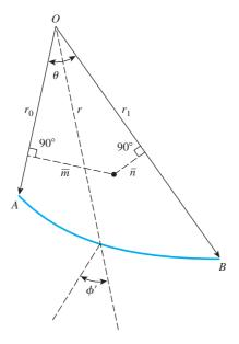
Figure 14.2 General parameters of a logarithmic spiral
