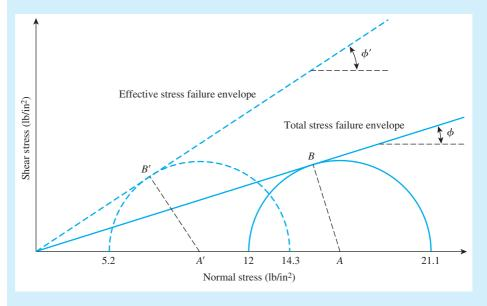
Figure 12.30 Failure envelopes and Mohr's circles for a saturated sand
