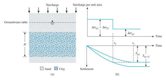
Figure 11.39 Principles of precompression
