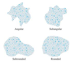
Figure 2.29 Shape of bulky particles
