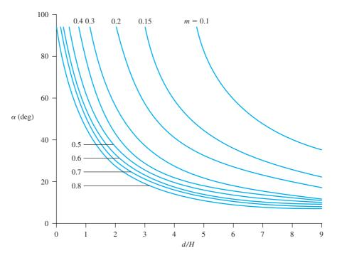
Figure 8.14 Chart for solution by L. Casagrande's method based on Gilboy's solution
