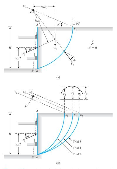
Figure 14.10 Determination of active force on bracing system of open cut in cohesionless soil
