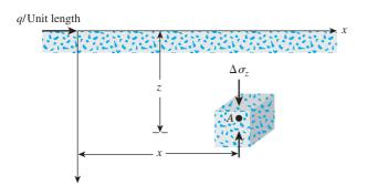
Figure 10.10 Horizontal line load over the surface of a semi-infinite soil mass
