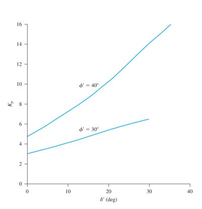
**Figure 14.4** Variation of  $K_p$  with  $\phi'$  and  $\delta'$  based on the procedure of Terzaghi and Peck (1967) (*Note*:  $\theta = 0$ ) (*Based on Terzaghi and Peck*, 1967)
