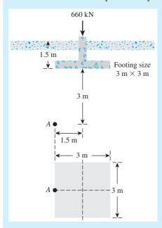
**Figure 10.28** Cross section and plan of a column footing
