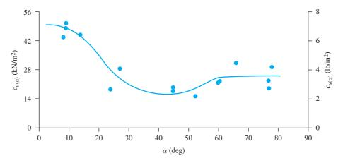
*Figure 12.42* Directional variation of  $c_u$  for undisturbed Winnipeg Upper Brown clay (*Based on Loh and Holt, 1974*)
