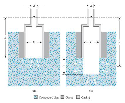
Figure 7.23 Permeability test with Boutwell permeameter
