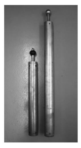
Figure 6.7 Comparison between standard Proctor hammer (left) and modified Proctor hammer (right) (Courtesy of Braja M. Das, Henderson, Nevada)
