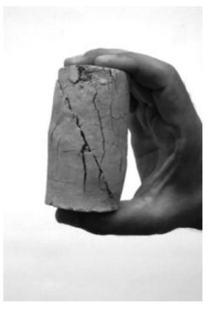
Figure 12.35 Failure by shear of an unconfined compression test specimen (Courtesy of Braja M. Das, Henderson, Nevada)
