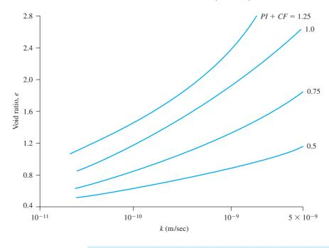
Figure 7.13 Variation of void ratio with hydraulic conductivity of clayey soils (Based on Tavenas, et al, 1983)
