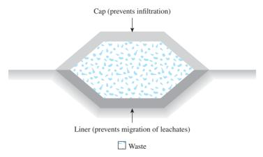
Figure 17.16 Landfill with liner and cap
