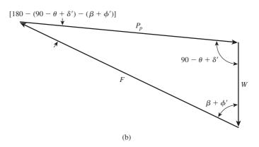
Figure 13.26 Coulomb's passive pressure: (a) trial failure
