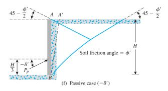
**Figure 14.1** Effect of wall friction on failure surface
