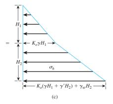
*Figure 13.5* Distribution of earth pressure at rest for partially submerged soil
