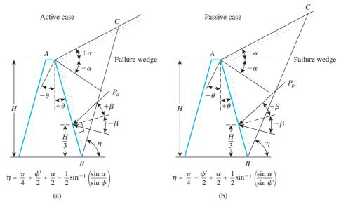
Figure 13.11 Location and direction of resultant Rankine force
