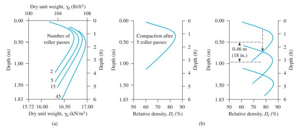
**Figure 6.20** (a) Vibratory compaction of a sand—variation of dry unit weight with number of roller passes; thickness of lift = 2.44 m (8 ft); (b) estimation of compaction lift thickness for minimum required relative density of 75% with five roller passes (*After D' Appolonia, Whitman, and D' Appolonia, 1969. With permission from ASCE.*)
