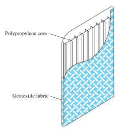
Figure 11.37 Prefabricated vertical drain (PVD)
