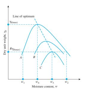
Figure 6.21 Most economical compaction condition
