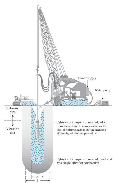
Figure 6.31 Vibroflotation unit (After Brown, 1977. With permission from ASCE.)
