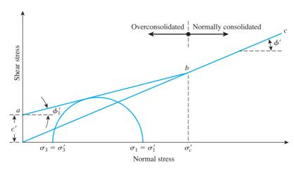
Figure 12.23 Effective stress failure envelope for overconsolidated clay
