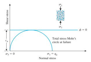
Figure 12.33 Unconfined compression test
