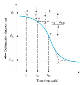
**Figure 11.25** Logarithm-of-time method for determining coefficient of consolidation
