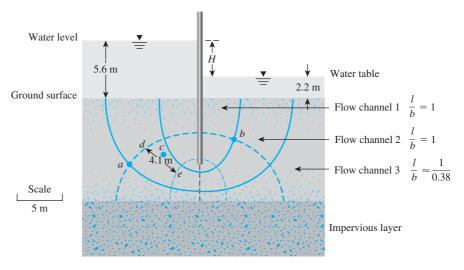
Figure 8.7 Flow net for seepage around a single row of sheet piles
