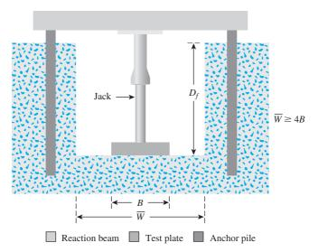
Figure 16.16 Diagram of plate load test
