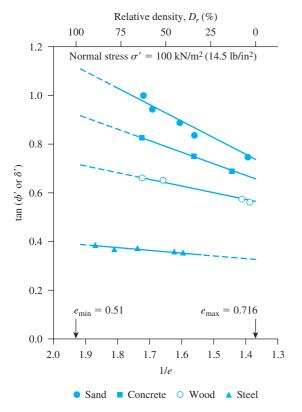
**Figure 12.15** Variation of  $\tan \phi'$  and  $\tan \delta'$  with 1/e [Note: e = void ratio,  $\sigma' = 100 \text{ kN/m}^2$  (14.5 lb/in.²), quartz sand] (After Acar, Durgunoglu, and Tumay, 1982. With permission from ASCE.)
