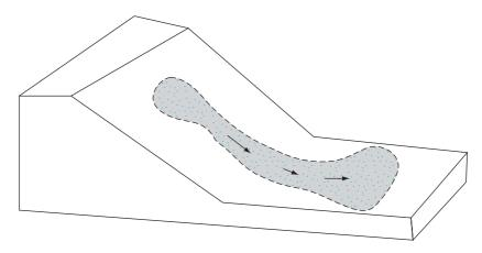
Figure 15.6 Slope failure by "flowing"
