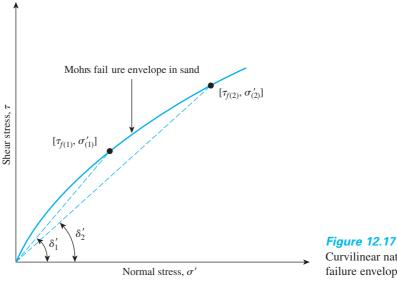
Curvilinear nature of Mohr's failure envelope in sand
