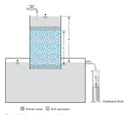
Figure 7.5 Constant-head permeability test
