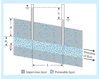
Figure 7.8 Flow through permeable layer
