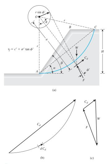
**Figure 15.22** Stability analysis of slope in homogeneous  $c'-\phi'$  soil
