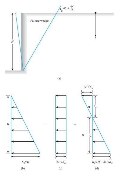
Figure 13.16 Rankine's active earth-pressure distribution against a retaining wall with cohesive soil backfill
