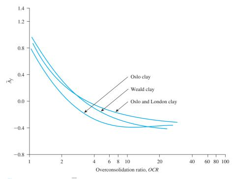
Figure 12.29 Variation of  $\overline{A}_f$  with overconsolidation ratio for three clays (Based on Simon, 1960)
