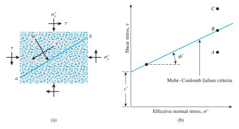
Figure 12.1 Mohr-Coulomb failure criterion
