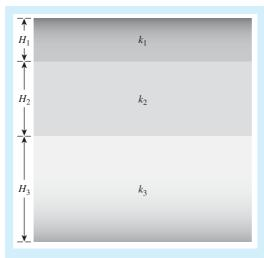
Figure 7.19 A layered soil profile
