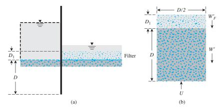
Figure 9.12 Factor of safety against heave, with a filter
