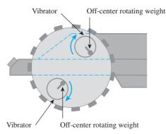
Figure 6.18 Principles of vibratory rollers
