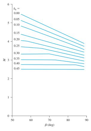
**Figure 15.20** Variation of M with  $k_h$  based on Koppula's analysis (for  $\beta \ge 55^{\circ}$ )
