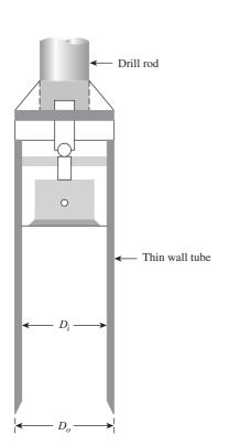
*Figure 18.8* Thin-wall tube sampler
