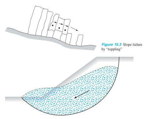
Figure 15.4 Slope failure by "sliding"
