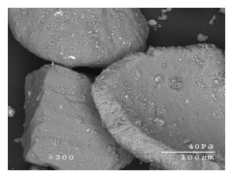
Figure 2.9 Higher magnification of the sand grains highlighted in Figure 2.8 (Courtesy of David J. White, Iowa State University, Ames, Iowa)
