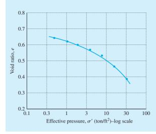
Figure 11.11 Variation of void ratio with effective pressure
