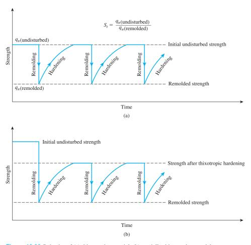
Figure 12.39 Behavior of (a) thixotropic material; (b) partially thixotropic material
