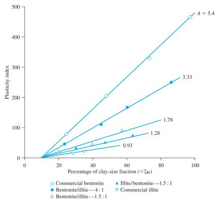
Figure 4.14 Relationship between plasticity index and clay-size fraction by weight for illite/bentonite clay mixtures (After Seed, Woodward, and Lundgren, 1964a. With permission from ASCE.)
