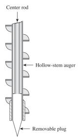
Figure 18.3 Schematic diagram of hollow-stem auger with removable plug
