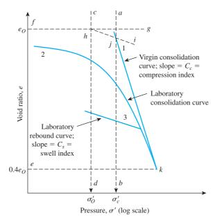
Figure 11.15 Consolidation characteristics of overconsolidated clay of low to medium sensitivity
