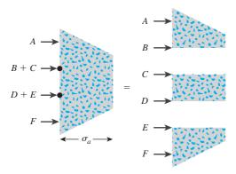
Figure 14.12 Determination of strut loads from empirical lateral pressure diagrams
