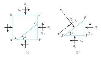
Figure 10.1 (a) A soil element with normal and shear stresses acting on it; (b) free body diagram of EFB as shown in (a)
