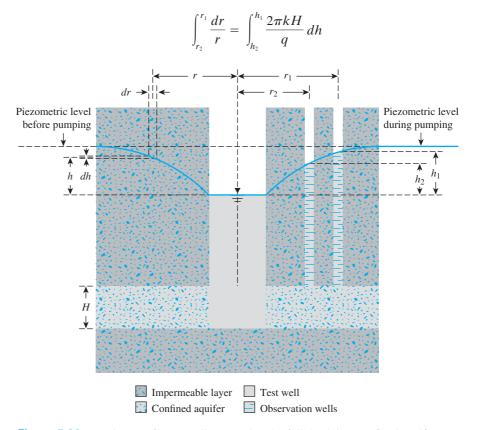
Figure 7.22 Pumping test from a well penetrating the full depth in a confined aquifer
