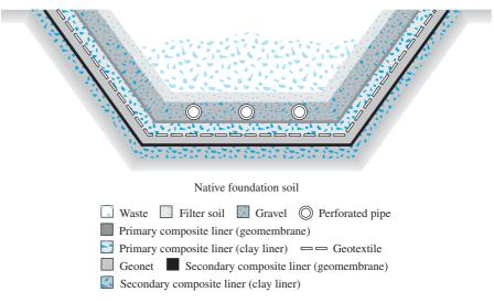
*Figure 17.11* Cross section of double-liner system (note the primary and secondary composite liners)
