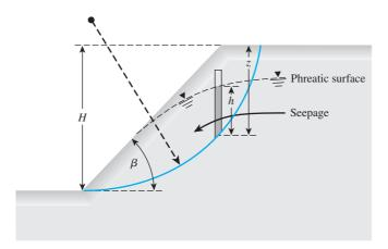
**Figure 15.34** Stability analysis of slope with steady-state seepage
