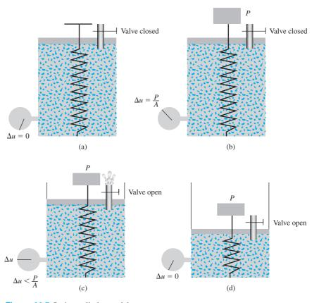
Figure 11.5 Spring-cylinder model
