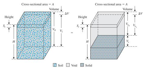
Figure 11.16 Settlement caused by one-dimensional consolidation
