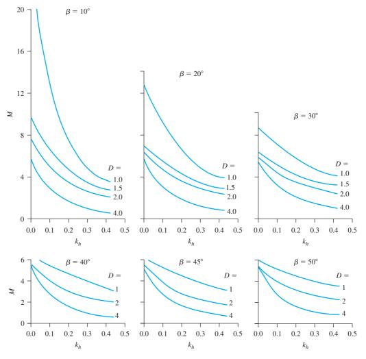
**Figure 15.19** Variation of M with  $k_h$  and  $\beta$  based on Koppula's analysis
