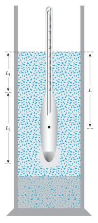
Figure 2.24 Definition of L in hydrometer test
