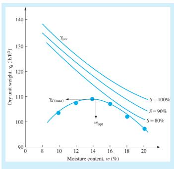
Figure 6.8 Moisture content-unit weight curves
