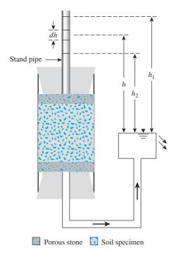
Figure 7.6 Falling-head permeability test
