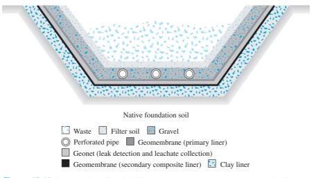
Figure 17.10 Cross section of double-liner system (note the secondary composite liner)
