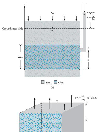
**Figure 11.22** (a) Clay layer undergoing consolidation; (b) flow of water at A during consolidation
