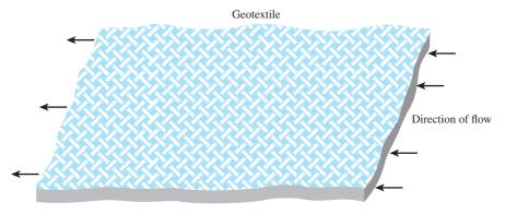
Figure 17.5 In-plane flow in geotextile
