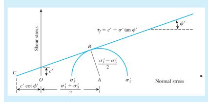
**Figure 12.56** Derivation of  $\alpha$  as a function of  $\phi'$  and m as a function of c' and  $\phi'$
