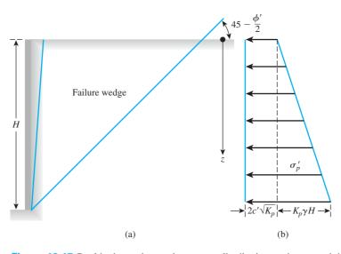
Figure 13.17 Rankine's passive earth-pressure distribution against a retaining wall with cohesive soil backfill
