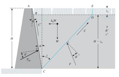
**Figure 13.30** Trial failure wedge behind a retaining wall with a  $c'-\phi'$  backfill
