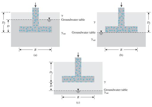
*Figure 16.6* Effect of the location of groundwater table on the bearing capacity of shallow foundations: (a) Case I; (b) Case II; (c) Case III
