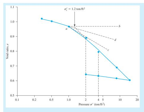
**Figure 11.17** Plot of e versus  $\log \sigma'$
