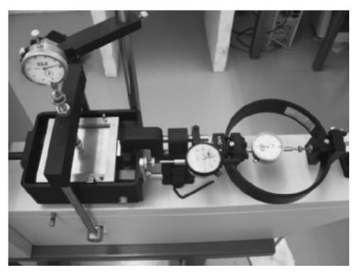
Figure 12.6 A photograph showing the dial gauges and proving ring in place (Courtesy of Braja M. Das, Henderson, Nevada)
