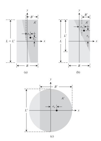
Figure 16.14 Foundation subjected to two-way eccentricity
