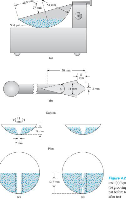
Figure 4.2 Liquid limit test: (a) liquid limit device; (b) grooving tool; (c) soil pat before test; (d) soil pat
