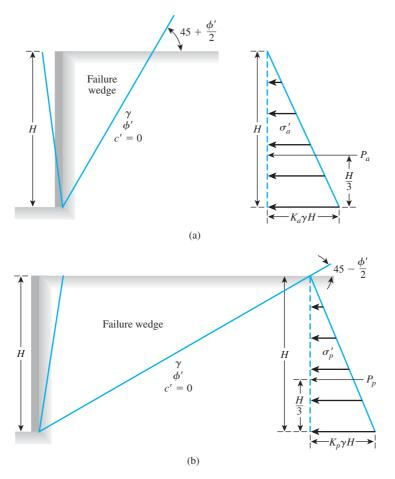
Figure 13.13 Pressure distribution against a retaining wall for cohensionless soil backfill with horizontal ground surface: (a) Rankine's active state; (b) Rankine's passive state
