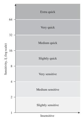
Figure 12.38 Classification of clays based on sensitivity
