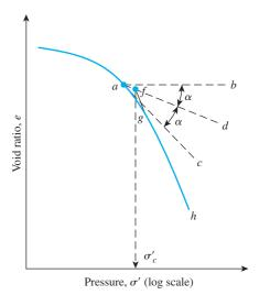
Figure 11.13 Graphic procedure for determining preconsolidation pressure
