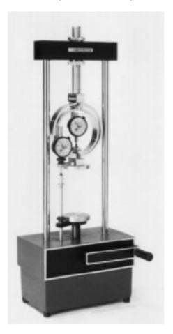
Figure 12.34 Unconfined compression test equipment (Courtesy of ELE International)
