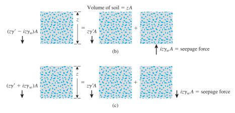
Figure 9.7 Force due to (a) no seepage; (b) upward seepage; (c) downward seepage on a volume of soil
