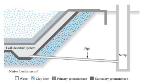
*Figure 17.15* Secondary LDCR system, by means of gravity monitoring. (*Note:* The plastic pipe penetrates the secondary geomembrane)
