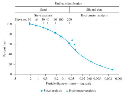
Figure 2.25 Particle-size distribution curve—sieve analysis and hydrometer analysis
