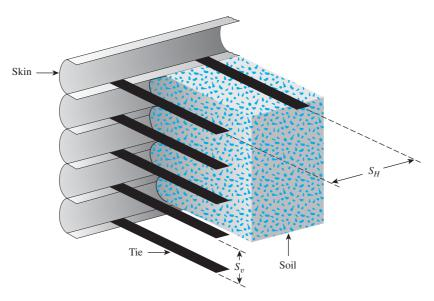
Figure 13.36 MSE wall with metallic strip reinforcement and metallic skin
