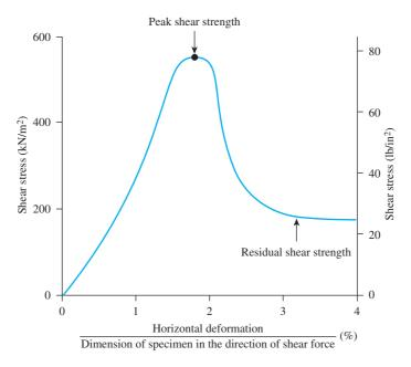
*Figure 12.10* Results of a drained direct shear test on an overconsolidated clay [*Note:* Residual shear strength in clay is similar to ultimate shear strength in sand (see Figure 12.7)]
