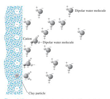
Figure 2.19 Attraction of dipolar molecules in diffuse double layer
