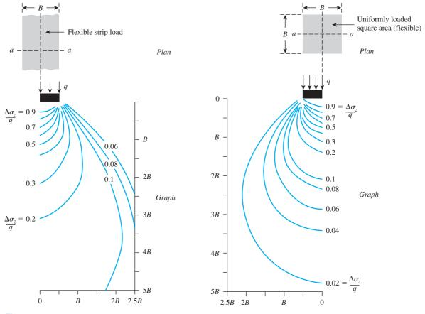
**Figure 10.25** Vertical pressure isobars under a flexible strip load (*Note*: Isobars are for line a-a as shown on the plan)
