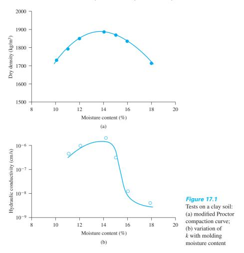
achieve the desired range of hydraulic conductivity. In addition, during field compaction, a heavy sheepsfoot roller can introduce larger shear strains during compaction that create a more dispersed structure in the soil. This type of compacted soil will have an even lower hydraulic conductivity. Small lifts should be used during compaction so that the feet of the compactor can penetrate the full depth of the lift.
