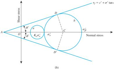
Figure 13.8 Rankine's passive earth pressure
