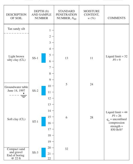
*Figure 18.15* Typical boring log (*Note:* SS = split-spoon sample; ST = Shelby tube sample)
