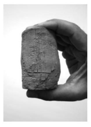
**Figure 12.36** Failure by bulging of an unconfined compression test specimen (Courtesy of Braja M. Das, Henderson, Nevada)
