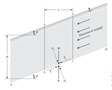
Figure 15.8 Infinite slope with steadystate seepage
