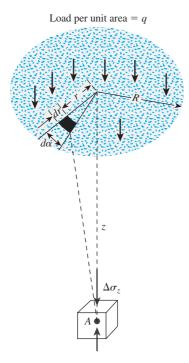
**Figure 10.17** Vertical stress below the center of a uniformly loaded
