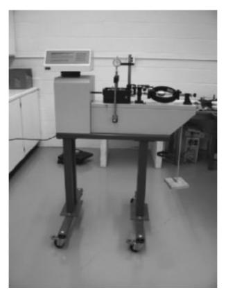
Figure 12.5 Strain-controlled direct shear equipment (Courtesy of Braja M. Das, Henderson, Nevada)
