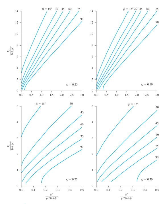
Figure 15.36 Michalowski's solution for steady-state seepage condition
