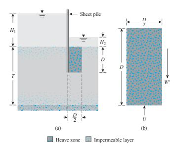
Figure 9.9 (a) Check for heaving on the downstream side for a row of sheet piles driven into a permeable layer; (b) enlargement of heave zone
