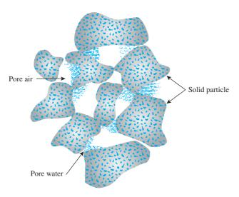
Figure 9.13 Partially saturated soil
