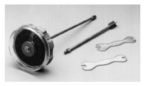
Figure 12.46 Laboratory vane shear test device (Courtesy of ELE International)
