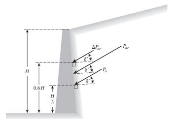
Figure 13.29 Location of the line of action of  $P_{ae}$
