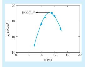
Figure 6.26 Plot of laboratorycompaction test results
