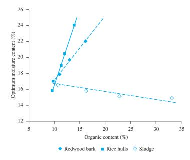
Figure 6.30 Variation of optimum moisture content with organic content — soil and organic material mixtures. (Source: After "The Effect of Organic Content on Soil Compaction," by J. Lancaster, R. Waco, J. Towle, and R. Chaney, 1996. In Proceedings, Third International Symposium on Environmental Geotechnology, p. 159. Used with permission of the author)
