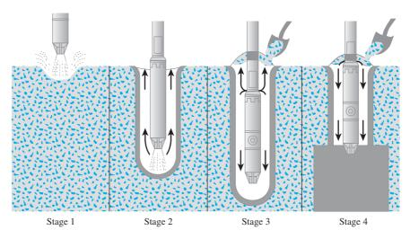
Figure 6.32 Compaction by vibroflotation process (After Brown, 1977. With permission from ASCE.)
