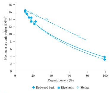
*Figure 6.29* Variation of maximum dry unit weight of compaction with organic content—soil and organic material mixture. (*Source:* After "The Effect of Organic Content on Soil Compaction," by J. Lancaster, R. Waco, J. Towle, and R. Chaney, 1996. In *Proceedings, Third International Symposium on Environmental Geotechnology*, p. 159. Used with permission of the author)
