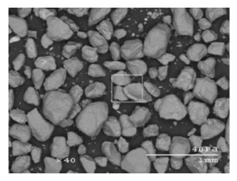
Figure 2.8 Scanning electron micrograph of some sand grains (Courtesy of David J. White, Iowa State University, Ames, Iowa)
