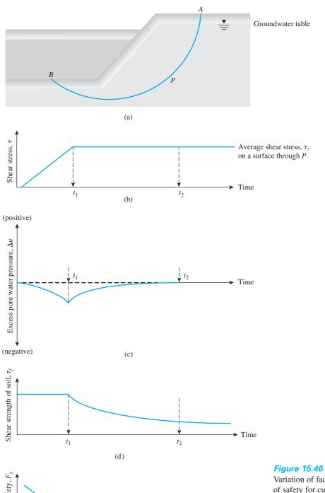
Variation of factor of safety for cut slope in soft clay (Redrawn after Bishop and Bjerrum, 1960. With permission from ASCE.)
