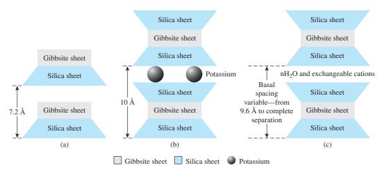
Figure 2.12 Diagram of the structures of (a) kaolinite; (b) illite; (c) montmorillonite
