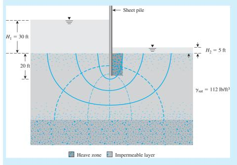
Figure 9.10 Flow net for seepage of water around sheet piles driven into permeable layer
