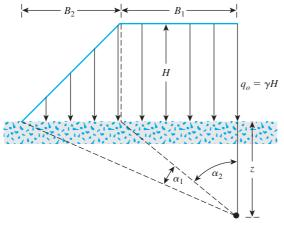
Figure 10.14 Embankment loading
