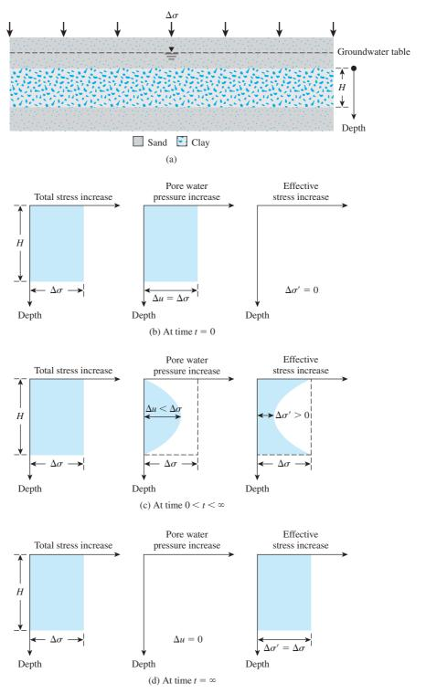
*Figure 11.6* Variation of total stress, pore water pressure, and effective stress in a clay layer drained at top and bottom as the result of an added stress,  $\Delta \sigma$
