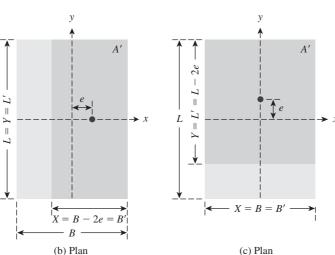
Figure 16.13 Ultimate load for shallow foundation under eccentric load
