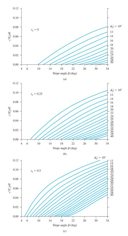
**Figure 15.35** Spencer's solution—plot of  $c'/F_s \gamma H$  versus  $\beta$
