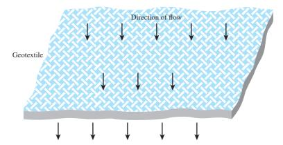
Figure 17.4 Cross-plane flow through geotextile
