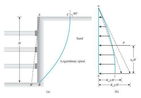
Figure 14.9 Earth-pressure distribution against a wall with rotation about the top
