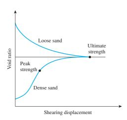
**Figure 12.8** Nature of variation of void ratio with shearing displacement
