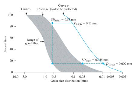
Figure 8.17 Determination of grain-size distribution of filter using Eqs. (8.41) and (8.42)
