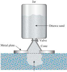
Figure 6.23 Field unit weight determined by Hole filled with Ottawa sand sand cone method
