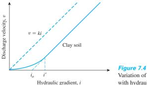
Variation of discharge velocity with hydraulic gradient in clay
