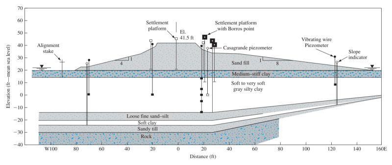
Figure 15.38 Cross-section through the centerline of the experimental test section looking north (After Ladd, 1972. With permission from ASCE.)
