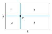
**Figure 10.22** Increase of stress at any point below a rectangularly loaded flexible area
