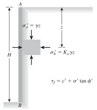
Figure 13.3 Earth pressure at rest
