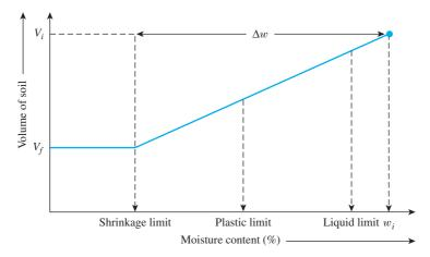
Figure 4.9 Definition of shrinkage limit
