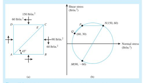
Figure 10.6 (a) Soil element with stresses acting on it; (b) Mohr's circle
