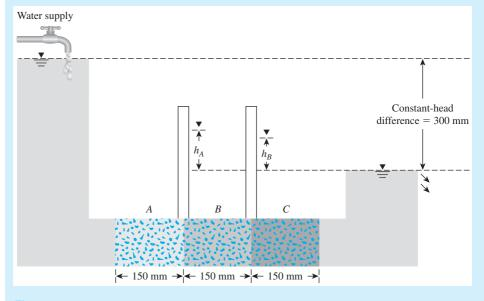
Figure 7.20 Three layers of soil in a tube 100 mm  $\times$  100 mm in cross section
