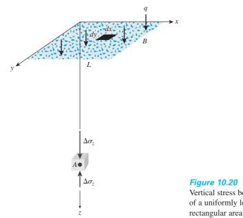
**Figure 10.20** Vertical stress below the corner of a uniformly loaded flexible
