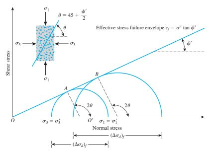
Figure 12.22 Effective stress failure envelope from drained tests on sand and normally consolidated clay
