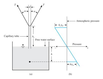
Figure 9.15 (a) Rise of water in the capillary tube; (b) pressure within the height of rise in the capillary tube (atmospheric pressure taken as datum)
