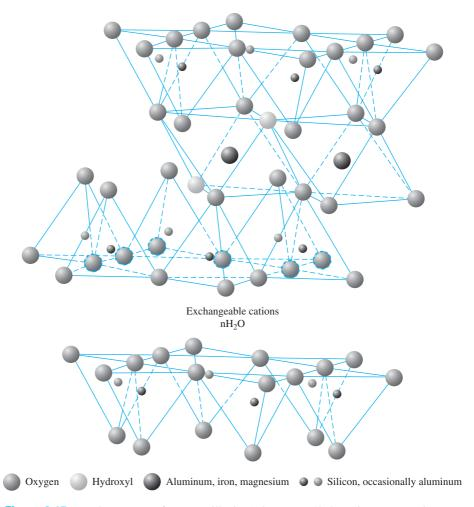
Figure 2.15 Atomic structure of montmorillonite (After Grim, 1959. With permission from ASCE.)
