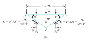
Figure 16.5 Terzaghi's bearing capacity analysis
