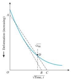
Figure 11.26 Square-root-of-time fitting method
