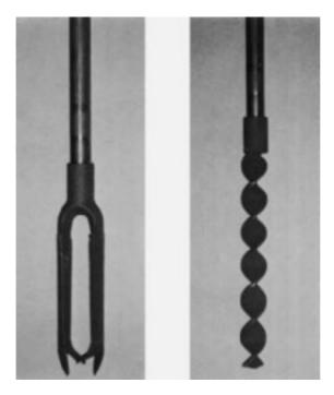
Figure 18.1 Hand augers: (a) Iwan auger; (b) slip auger (Courtesy of Braja M. Das, Henderson, Nevada)
