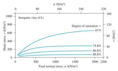
*Figure 12.52* Variation of the total stress failure envelope with change of initial degree of saturation obtained from undrained tests of an inorganic clay (*After Casagrande and Hirschfeld*, 1960. With permission from ASCE.)
