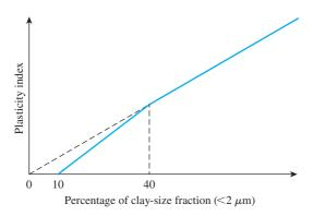
Figure 4.15 Simplified relationship between plasticity index and percentage of clay-size fraction by weight (After Seed, Woodward, and Lundgren, 1964b. With permission from ASCE.)
