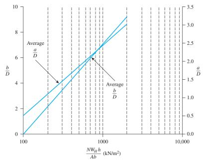
Figure 6.36 Poran and Rodriguez chart for a/D, b/D versus NW<sub>H</sub>h/Ab
