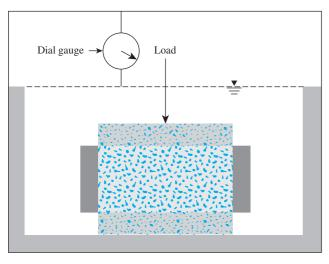
Porous stone Soil specimen Specimen ring
